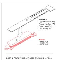
must be selected to make a complete actuator system. When selecting an appropriate actuator, please refer to the data sheets for both the NanoMuscle Motors and Interfaces.
