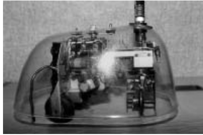
Figure 2.1 One of the tortoise robots built by W. Grey Walter. (Photo courtesy of Dr. Owen Holland)
