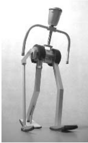
Figure 4.1 A passive walker: a robot that uses gravity and clever mechanics to balance and walk without any motors. (Photo by Jan van Frankenhuyzen, courtesy of Delft University of Technology)
