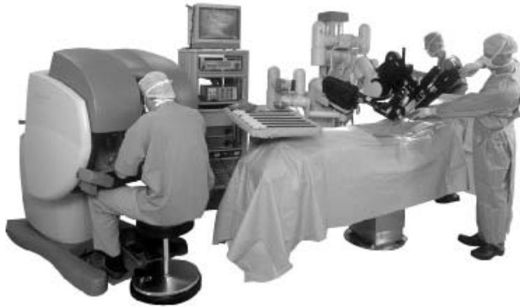
Figure 6.1 A complex teleoperated manipulator robot used in robot-assisted surgery in some hospitals. (Photo ©[2007] Intuitive Surgical, Inc.)
