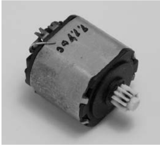
Figure 4.2 A standard direct-current (DC) motor, the most common actuator used in robotics.
