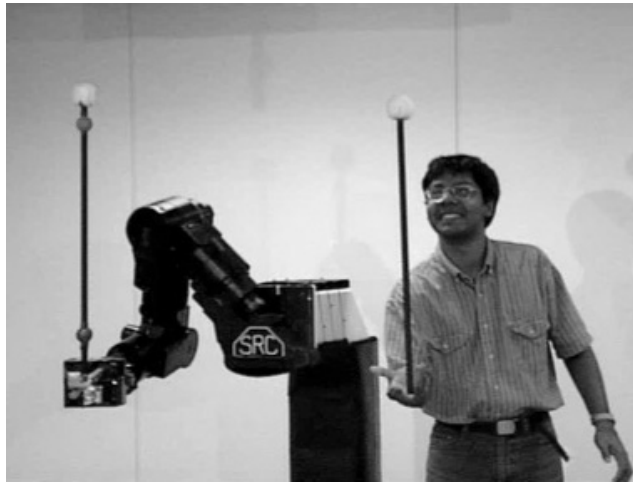
Figure 21.4 A humanoid robot learning to balance a pole by watching a human teacher. (Photo courtesy of Dr. Sethu Vijayakumar)
