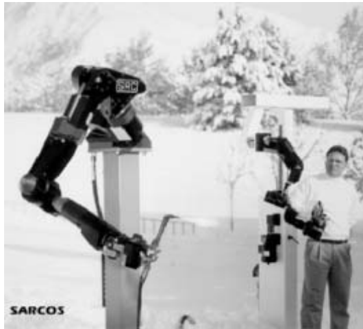
Figure 4.7 A humanlike seven DOF arm and an exoskeleton for teleoperating it. Both are made by Sarcos. (Photo courtesy of Sarcos Inc.)
