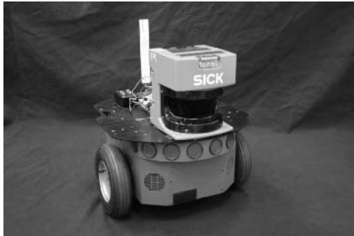
Figure 9.3 A mobile robot sporting a laser sensor. The laser is the thing that resembles a coffee maker and is labeled with the name of the manufacturer, SICK.
