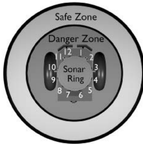
Figure 14.2 Sonar ring configuration and the navigation zones for a mobile robot.
