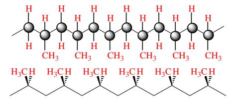
Figure 10.3 Isotactic polypropylene.
