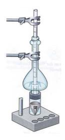
An instrument used to measure melting point.
