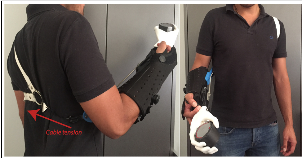
Figure 4. Our 3D-printed prosthetic hand attached to the simulator and a figure-of-nine shoulder harness. The cable tension that is delivered by the harness and activates the prosthetic hand is depicted (left).
