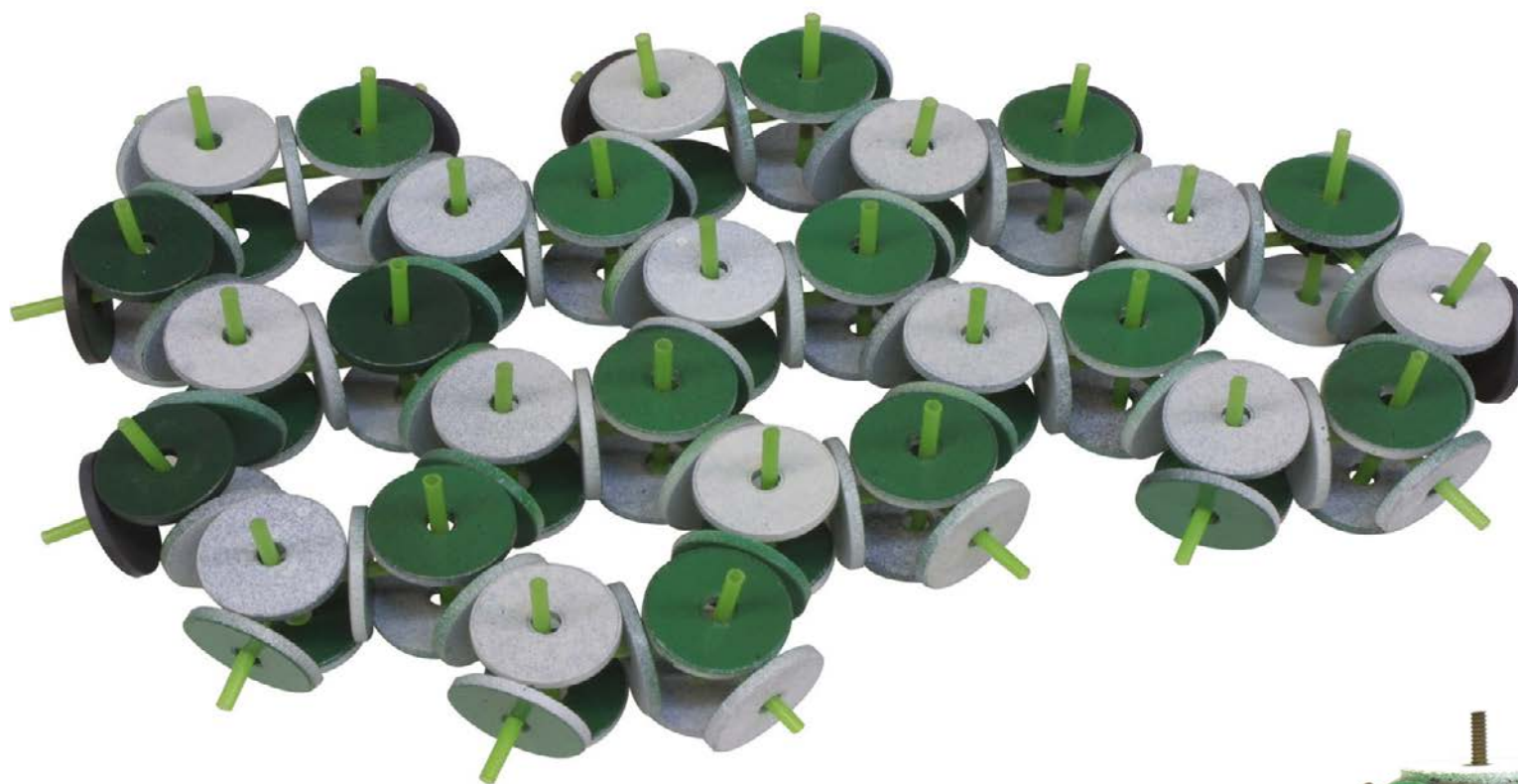
5-magnet cells in a hexagon beehive pattern. Magnetic linkage is continuous. In my atom model, this hexagon formation represents the arrangement of carbon atoms in a plane of graphene.
