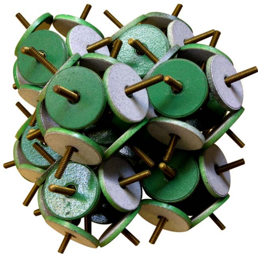
A body-centered array of 8-magnet spheres. If this pattern is extended indefinitely each 8-magnet unit will have 8 neighbors at its corner positions.
