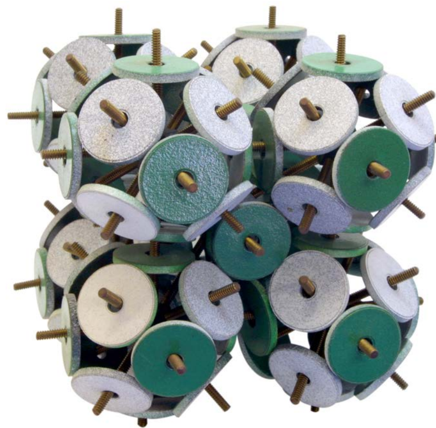
A body-centered cubic arrangement of 14-magnet spheres. Each sphere connects to its neighbors at the corner positions of a cube.
