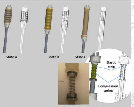
Actuator shown in different states. In state A the actuator works as an extensor while in state C the actuator works as a contractor. In state B the actuator stiffen only upon actuation. A close-up of the internal components is also shown.
