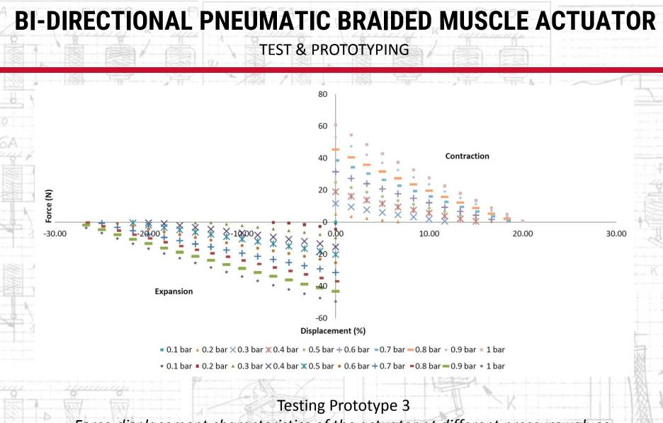
Force-displacement characteristics of the actuator at different pressure values. (x axis : displacement %, yaxis: force)
