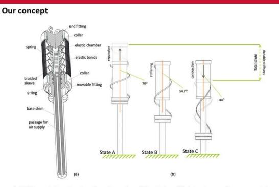
(a) CAD rendering showing the schematics of the design. (b) Actuator working concept. A single braid fiber is shown instead of the whole outer braided sleeve for clarity. State A
