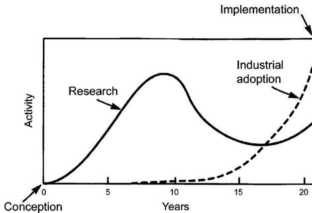
Fig. 1. Schematic of development history for new construction materials [2].
