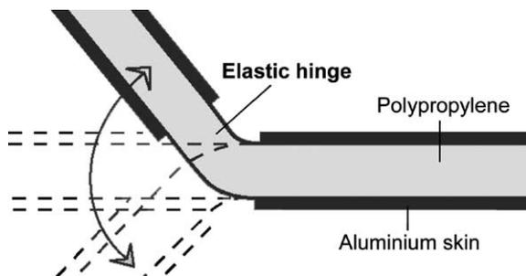
Fig. 3. Elastic hinge of Hylite.
