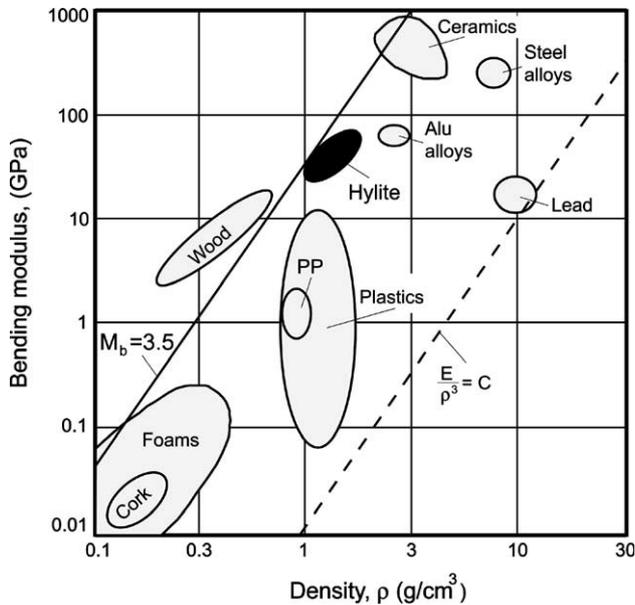
Fig. 2. Bending modulus plotted against density for lightweight, high stiffness design [8].
