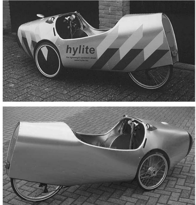
Fig. 9. H-Alleweder Velomobile with body made of Hylite.
