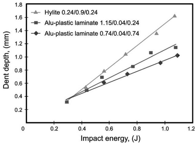
Fig. 6. Dynamic dent resistance of some aluminium plastic laminates.
