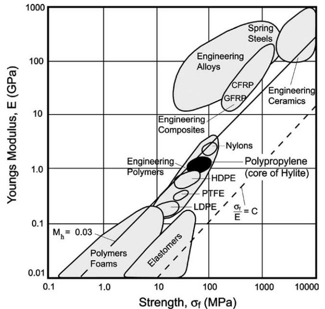
Fig. 4. Materials for elastic hinges [7].
