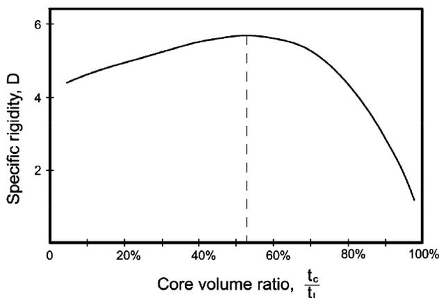
Fig. 5. Maximizing the specific rigidity of Hylite by varying the core volume ratio.
