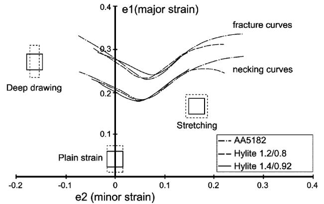
Fig. 7. FLD of Hylite (different thicknesses) and aluminium alloy.
