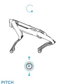
Y axis of right joystick changes robot's pitch (body angle)
