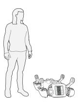
1. Stand to one side of Spot. Make sure motors are locked out.
