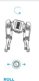
X axis of left joystick rolls robot's body
