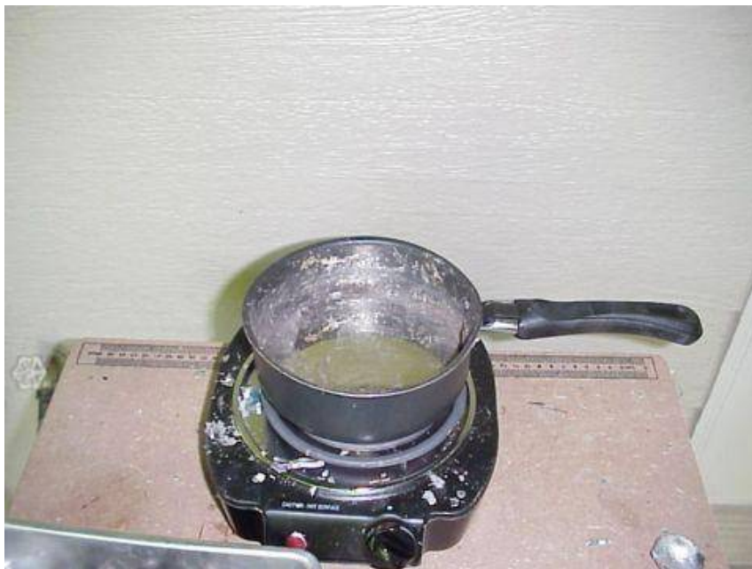
Clean alloy, ready for casting into ingots or bullets.
