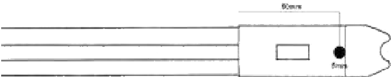
Position to drill catch hole in STEN magazine
