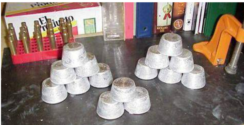
Filling the condiment cups about 2/3rds full results in convenient, 1 pound ingots.
