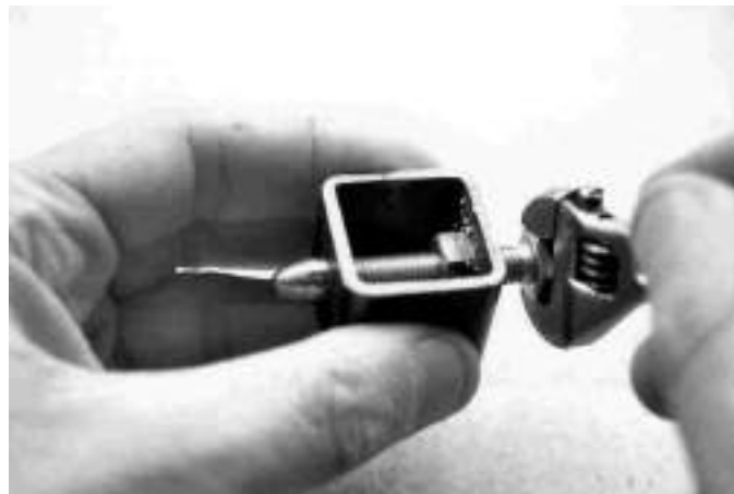
Press the bullet through the die.
