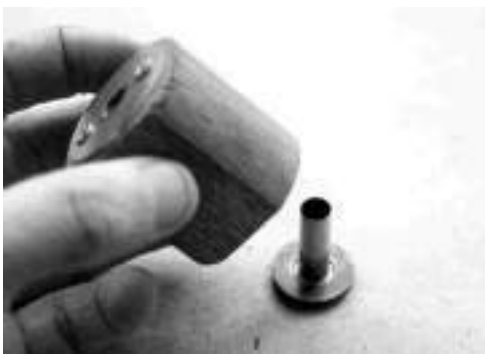
Insert the die over the case.
