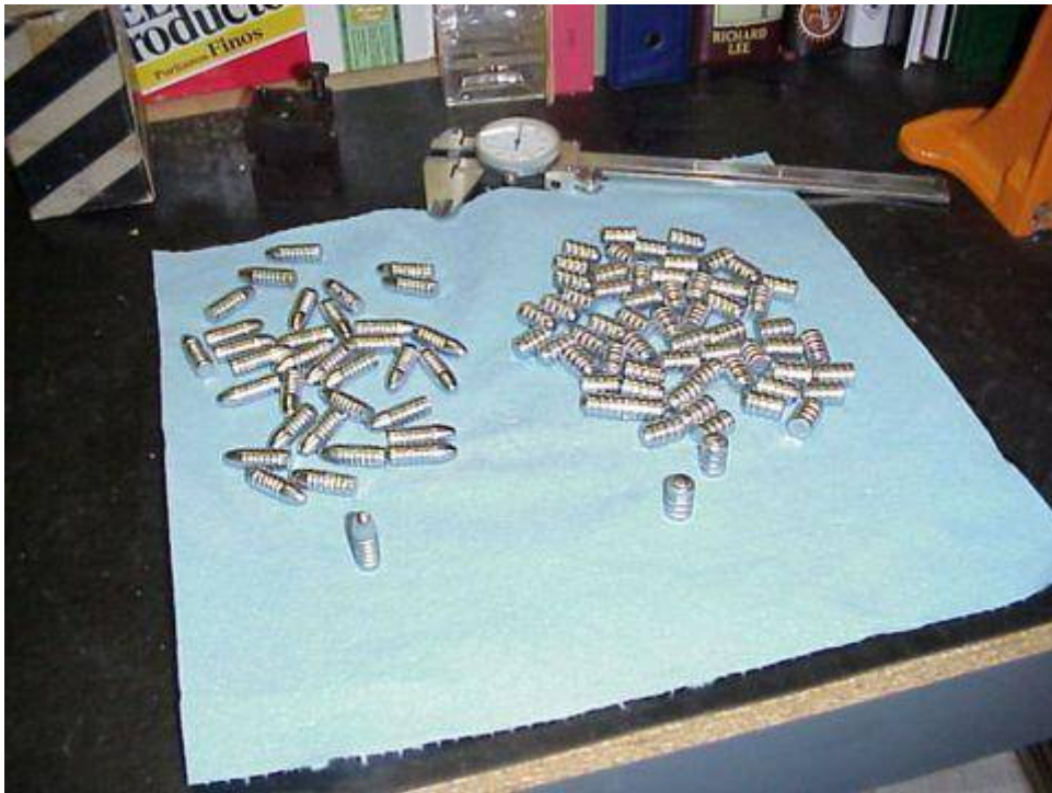
Some of my cast bullets: .314 rifle bullets on the right, and .357 wadcutters for my .38 special.
