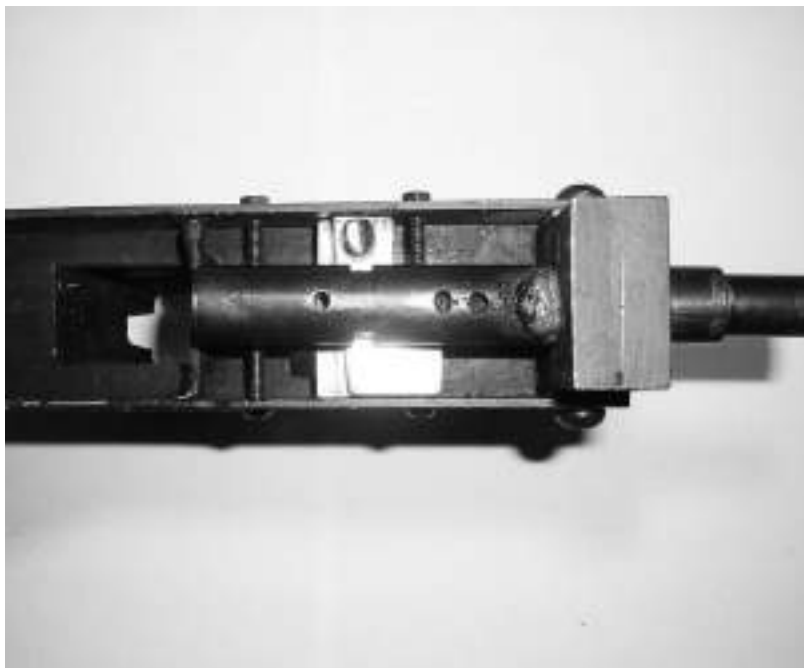
Destroyed dummy barrel of demonstration model
