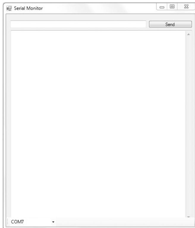
The screen elements are a textbox for data entry, a command button to send the entry to the Arduino, and another larger text box to display the data coming from the Arduino. Last, but not least, there is a combobox displaying all available USB COM ports (It is your task to determine the proper USB port; there is no auto detection).
