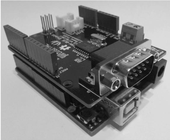
In terms of CAN capabilities, the shield by Seeek Studio provides the same functionality as the one by SK Pang electronics, however, it comes with a much lower price tag, because it does not have any additional components besides the CAN interface.
