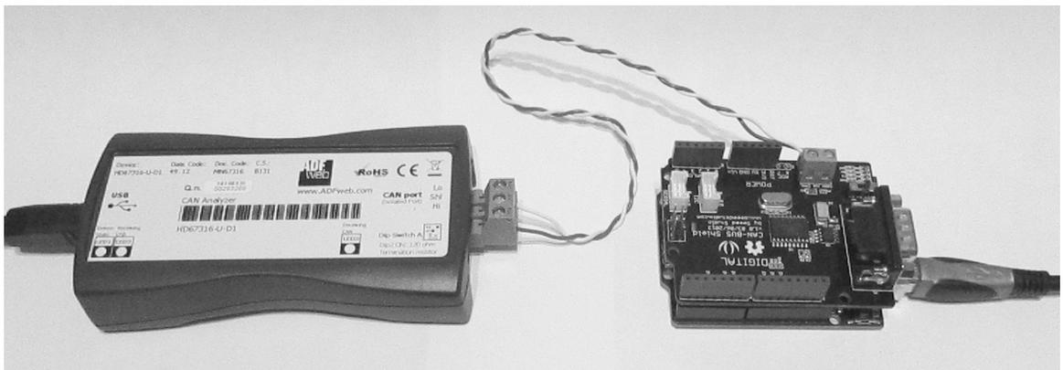
In order to test and verify the proper transmission and reception of CAN messages, I used the ADFweb CAN-to-USB gateway with its Windows interface.
