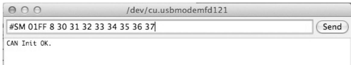
While the basic functionality of sending and receiving CAN messages remains the same, the program size and complexity has, naturally, grown. Most of the code, however, is being used for conversion between hex and ASCII formats (for readability) and some rudimentary syntax check.
