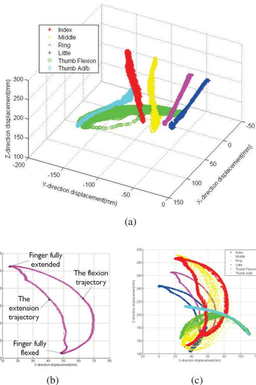
Fig. 10. The trajectories of the fingertips of our biomimetic robotic hand. (a) 3D scatter plot of fingertip trajectories. (b) The ring fingertip’s trajectories projected onto the X-Z plane. (Note: The scatter plot is from the 20 repetitions of the full flexion and extension motions.) (c) The trajectories of the fingertips projected onto the X-Z plane.
