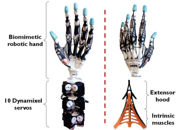
Fig. 1. The fully assembled biomimetic robotic hand. *Left*: The palmar aspect of the biomimetic robotic hand system. *Top right*: The dorsal view of the robotic hand. *Bottom right*: The laser-cut extensor hood integrated with intrinsic muscles. *Note*: The total weight of our biomimetic robotic hand is less than 1 kg (942 grams) including the actuation system.
