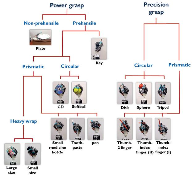
Fig. 12. The hand taxonomy realized by our biomimetic robotic hand (Note: see the taxonomy figure in [22] for comparison).
