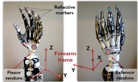
Fig. 8. Labeled pictures showing the differential pulley transmission for ring and little fingers and the locations of the reflective markers. *Note:* All the marker coordinates were recorded with respect to the forearm frame.
