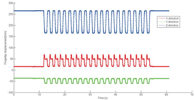
Fig. 9. The displacement of the ring's fingertip during 20 repetition of flexion and extension motions. *Note:* Similar tracking data were recorded and observed for the little finger.
