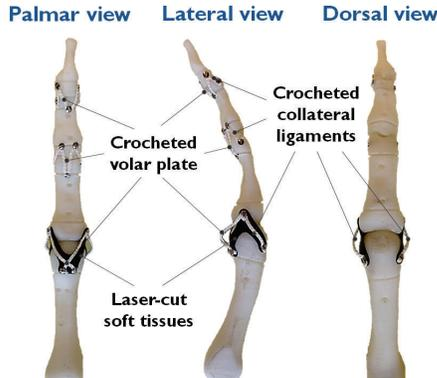
Fig. 5. The skeleton of the 3D-printed finger connected by crocheted ligaments and laser-cut joint soft tissues. *Note:* All the crocheted ligaments are anchored by 1 mm screws at their biological insertion sites.
