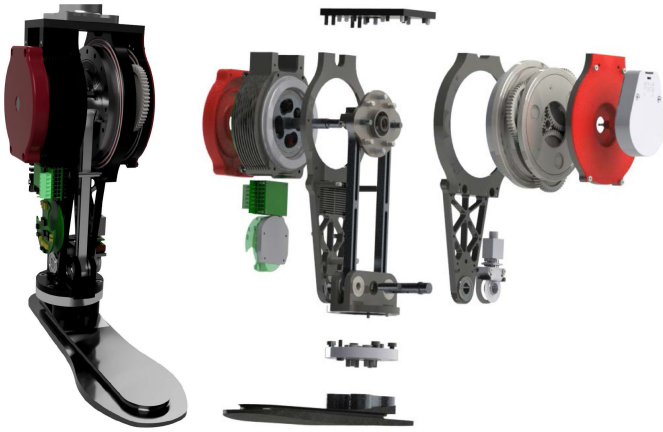
Fig. 6. CAD design of the ankle actuator. The image on the left-hand side presents the assembled ankle actuator. The exploded view on the right-hand side displays the components/subassemblies of the ankle actuator, such as the motor, structure, four-bar linkage, transmission, electronics, and foot.
