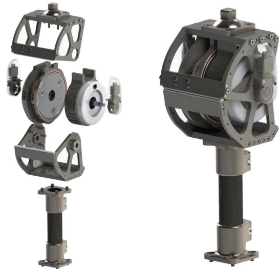
Fig. 5. CAD design of the knee actuator. The exploded view on the left-hand side displays the components/subassemblies of the knee actuator, such as the upper/lower hinges, encoders, transmission, motor, and pylon. The image on the right-hand side presents the assembled knee actuator. The pyramid adapter on top connects to the user's socket, and the length-adjustable pylon on bottom connects to the ankle actuator module.
