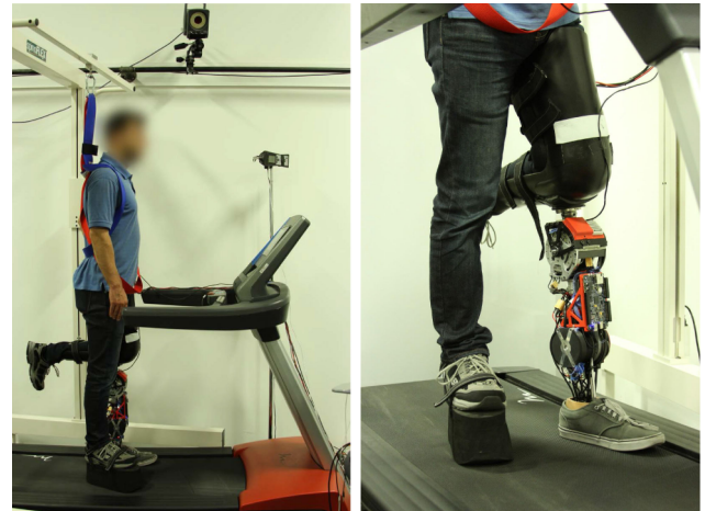
Fig. 14. Experimental setup for AB walking experiments. The image on the left-hand side shows the subject, safety harness, treadmill, and sound-level meter. The image on the right-hand side shows how the PR leg was connected to the bypass adapter, and how it was attached to the subject's leg.
