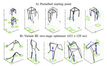
Fig. 6: Sensitivity of the joint-space model to initial conditions. (A) The starting points are only slightly different, (B) but the optimization seems very sensitive, converging to different local minima (two trials per task). Here we used variant III optimization with same parameters as Figure.5. The vector-based model converges to the same solution every time, not interesting to show.
