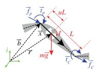
Fig. 2: Notations used to model a segment of the robot by vectors in the inertial frame. The unitary vector  $\vec{x}$  represents the segment alignment expressed in the inertial frame as well as the interaction forces and torques (shown in blue). Model-specific parameters are also shown in red.
