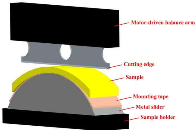
Figure 1. Schematic diagram of the cutting test.
