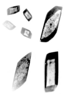
**Figure 7.67.** Photographs of NaHZn  $(P_2O_7)$  crystals (magnification  $\times$  30).[301]
