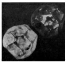
Figure 9.25. In<sub>3</sub>Sb<sub>5</sub>O<sub>12</sub> crystals obtained under hydrothermal conditions.<sup>[108]</sup>
