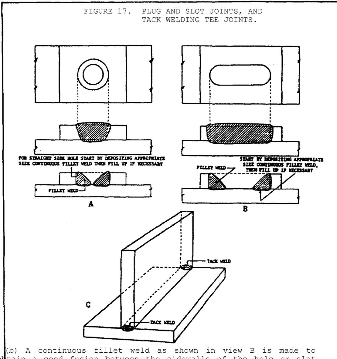
(b) A continuous fillet weld as shown in view B is made to obtain a good fusion between the sidewalls of the hole or slot and the surface of the lower plate. The procedure for this fillet weld is the same as for lap joints, which will be described in paragraph 5g(2) on page 45. The hole or slot is then filled in to provide additional strength in the weld.
