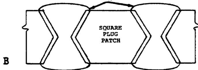
DOUBLE BEVEL, PATCH AND SIDEWALLS OF HOLE
