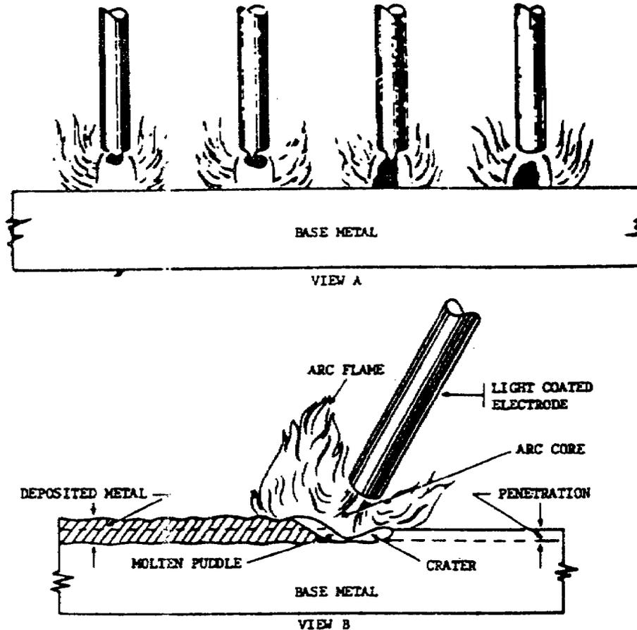
(c) Some of the light coatings may produce a slag, but it is quite thin and does not act in the same manner as the shielded-arc, slag-type electrode. The action of an arc obtained with a light-coated electrode is shown in figure 1, view B.
