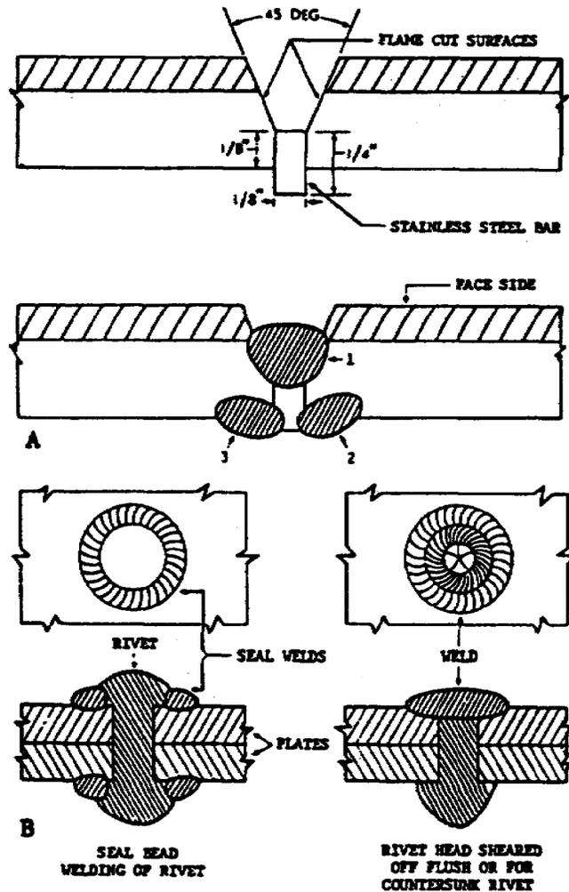
by 1/4 inch stainless steel bar which is placed in the damaged portion of the armor plate. It is then bead welded in place. The principal advantages of this joint are its simplicity, and good structural and ballistic properties. Care should be taken that no welding is done on the hard face side of the armor plate.
