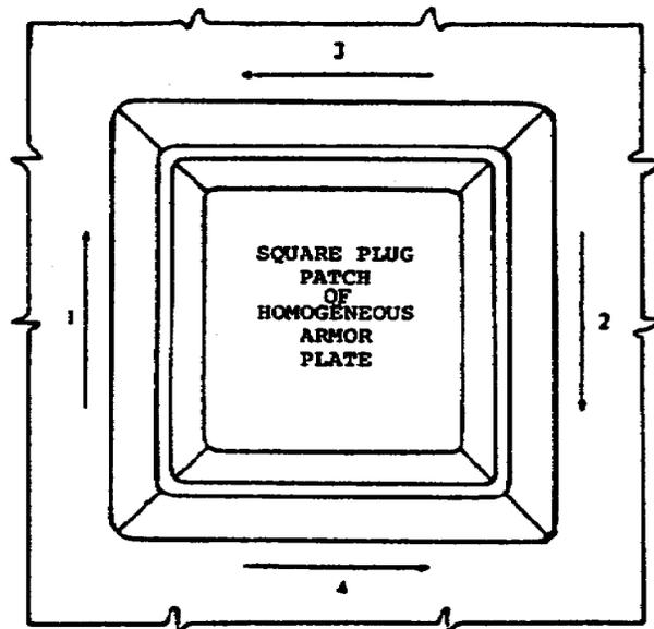
SQUARE PLUG DESIGN HAS DISTINCT ADVANTAGES OVER ROUND PLUG IN THAT STRAIGHT LINE WELDS CAN BE MADE. ROUND PLUGS REQUIRE CONSTANT VARIATION IN ANGLE OF ELECTRODE TO MAKE CURVED WELDS. THIS PROCEDURE PROMOTES ERRATIC PENETRATION AND IRREGULAR WELDS. NUMBERS INDICATE SEQUENCE TO BE USED IN WELDING
