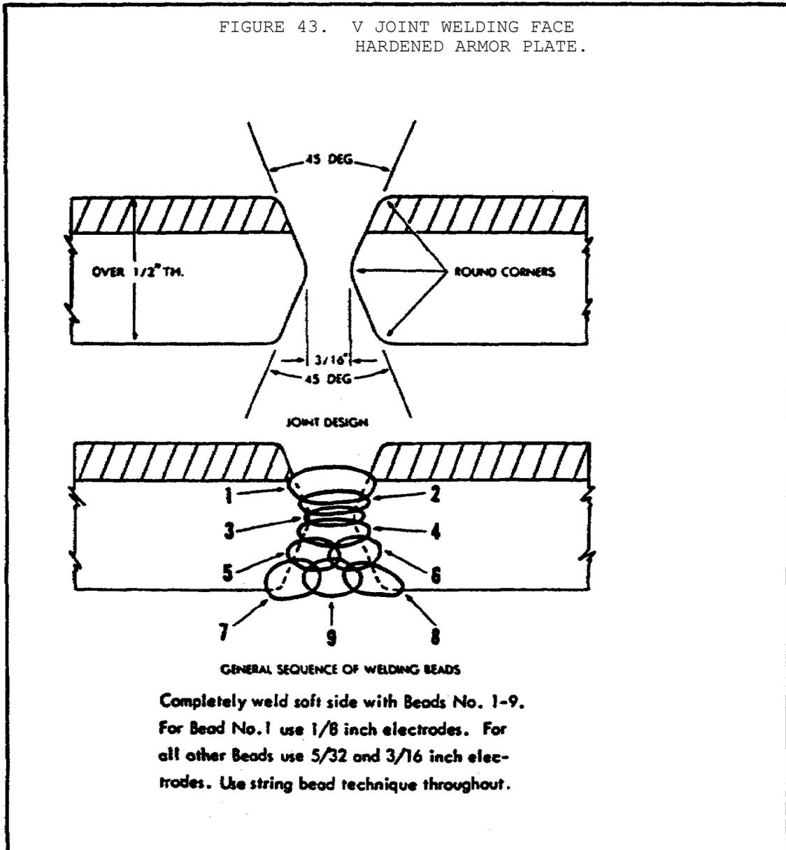
completely welded before welding on the face side. Using string bead welds, and the backstep and overlap procedures for the root passes, reduces the danger of cracks developing in the weld. To keep the structure free of warpage, no weaving motion of the welding rod should be used on this type joint.
