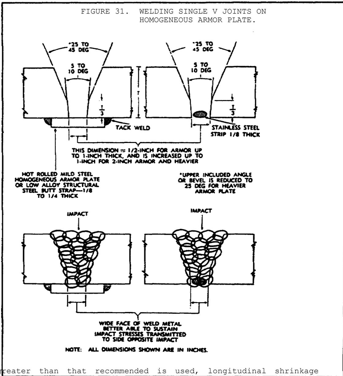
greater than that recommended is used, longitudinal shrinkage cracks in the weld or fusion zone may develop.
