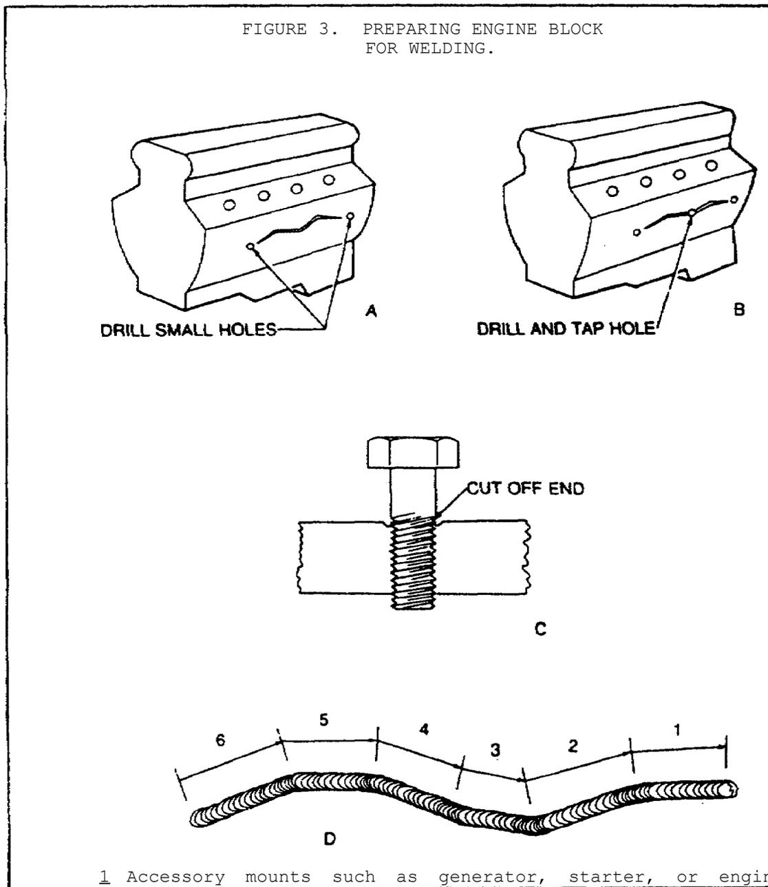
1 Accessory mounts such as generator, starter, or engine mounts. Because of possible warpage, mount alignment must be checked after welding.
