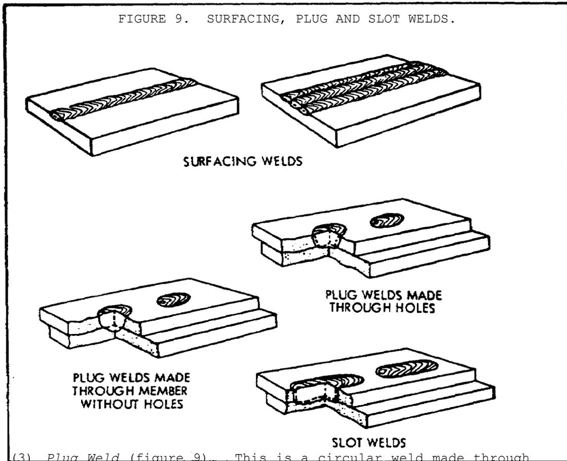
(3) *Plug Weld* (figure 9). This is a circular weld made through one member of a lap or tee joint joining that one member with the other. This type weld may or may not be made through a hole in the first member.
