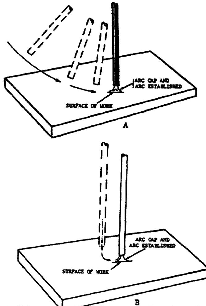
(2) In the striking and brushing method, the electrode is brought down to the work with a lateral motion similar to that of striking a match. As soon as the electrode touches the work surface, the electrode is raised to establish the arc. The arc length or gap between the end of the electrode and the work should be approximately equal to the diameter of the electrode. When the proper length of the arc is obtained, a sharp crackling sound can be heard.
