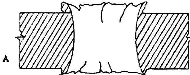
SHELL PENETRATION IN HOMOGENEOUS ARMOR PLATE. ALL TORN AND IRREGULAR EDGES SHOULD BE FLAME CUT BEFORE BEVELING SIDEWALLS FOR WELDING
