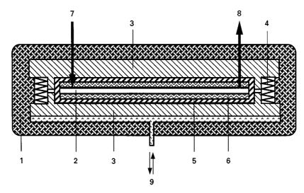
Figure 2 Schematic diagram of online OPLC. 1, Support block; 2, chromatoplate; 3, support plate; 4, spring; 5, casette system for fixing the chromatoplate between two Teflon layer; 6, Teflon layer; 7, Mobile phase inlet; 8, mobile phase outlet; 9, hydraulic system.
