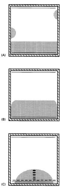
**Figure 7** Elimination of typical problems in OPLC. (A) 'Break-in effect' – a consequence of improper impregnation of the chromatographic plate; (B) 'meniscus effect' – a consequence of improper impregnation of the chromatographic plate; (C) lack of the appropriate inlet pressure for linear separation.
