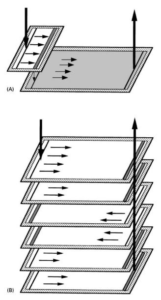
**Figure 6** Micropreparative ML-OPLC separations on analytical HPTLC plates. (A) Schematic diagram of cleanup procedure using fully online LD-OPLC; (B) schematic diagram of fully online LD-OPLC for a large amount of a complex mixture.
