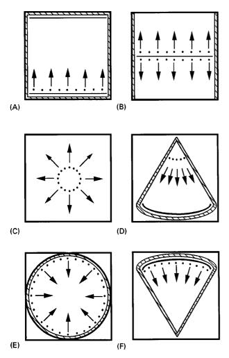
**Figure 5** Development modes in analytical OPLC using 20 cm  $\times$  20 cm HPTLC chromatographic plates. (A) Linear unidirectional; (B) linear two-directional; (C) circular with 8 cm development distance; (D) circular with 18 cm development distance, or online circular; (E) anticircular; (F) anticircular with 18 cm development distance, or online anticircular.
