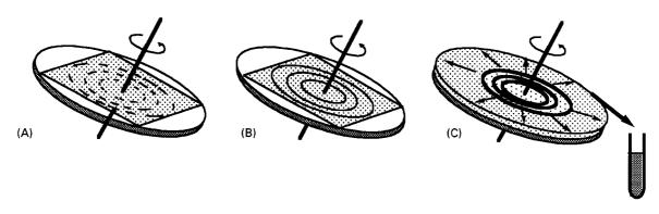
Figure 10 Principles of RPC. (A) Fully offline analytical separation; (B) fully offline micropreparative separation; (C) fully online preparative separation.
