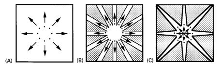
Figure 13 Development modes in analytical RPC on 20 cm × 20 cm HPTLC plates. (A) Circular; (B) linear; (C) anticircular.
