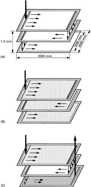
Figure 4 Schematic diagram of long-distance OPLC (LD-OPLC). (A) Principle of the method; (B) fully offline LD-OPLC using homolayers; (C) fully online LD-OPLC using heterolayers.
