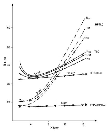
Figure 1 Comparison of the efficiency of analytical TLC and HPTLC chromatographic plates when used with capillary action and forced-flow planar chromatography (FFPC).  $N_{US}$ , normal unsaturated chamber; UM, ultramicrochamber;  $N_{US}$ , normal saturated chamber.
