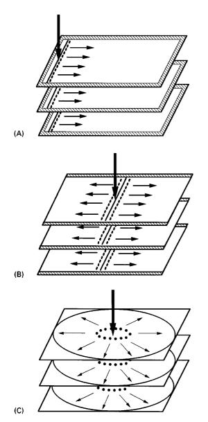
Figure 3 Schematic diagram of multi-layer OPLC (ML-OPLC). (A) Linear one-directional development; (B) linear two-directional development; (C) circular development.
