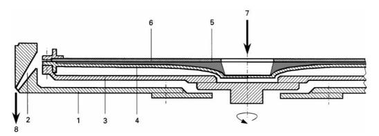
**Figure 12** Schematic diagram of preparative C-RPC. 1 = lower part of the stationary chamber, 2 = collector, 3 = motor shaft with the rotating disc, 4 = rotating planar column, 5 = stationary phase, 6 = quartz glass cover plate, 7 = mobile phase inlet, 8 = eluent outlet.
