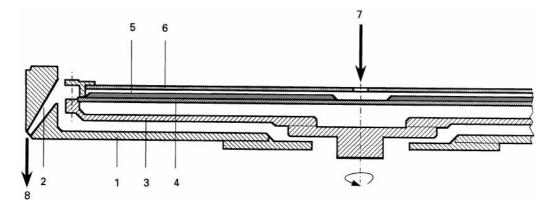
**Figure 11** Schematic diagram of preparative M-RPC. 1 = lower part of the stationary chamber, 2 = collector, 3 = motor shaft with the rotating disc, 4 = glass rotor, 5 = stationary phase, 6 = quartz glass cover plate, 7 = mobile phase inlet, 8 = eluent outlet.
