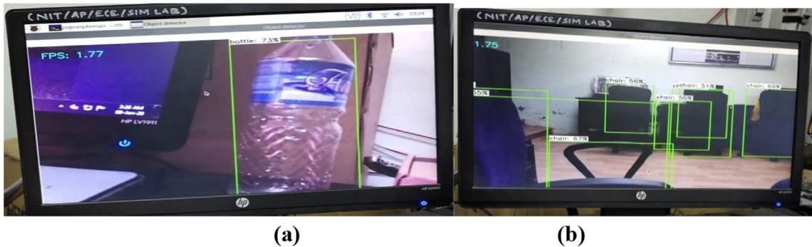
Fig. 7. (a) A water bottle is detected (b) chair is detected.
