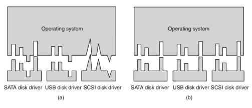
Figure 5-14. (a) Without a standard driver interface. (b) With a standard driver interface.
