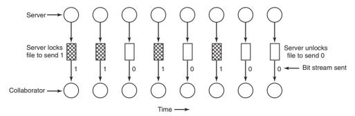
Figure 9-13. A covert channel using file locking.
