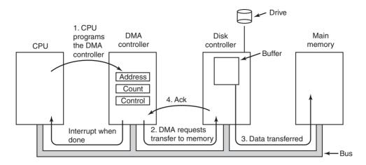
Figure 5-4. Operation of a DMA transfer.
