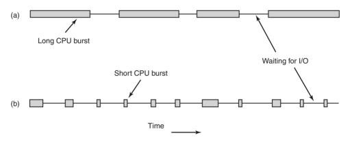
**Figure 2-39.** Bursts of CPU usage alternate with periods of waiting for I/O. (a) A CPU-bound process. (b) An I/O-bound process.
