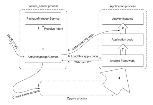
Figure 10-67. Steps in launching a new application process.
