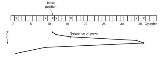
Figure 5-25. The elevator algorithm for scheduling disk requests.
