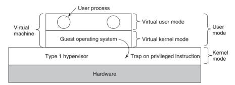
**Figure 7-3.** When the operating system in a virtual machine executes a kernel-only instruction, it traps to the hypervisor if virtualization technology is present.
