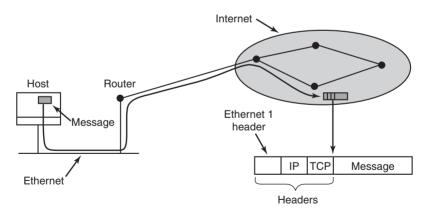
**Figure 8-31.** Accumulation of packet headers.
