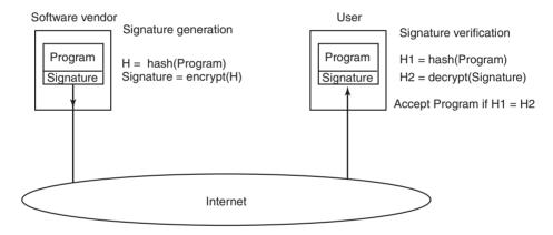
Figure 9-35. How code signing works.
