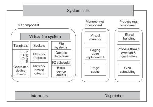
Figure 10-3. Structure of the Linux kernel
