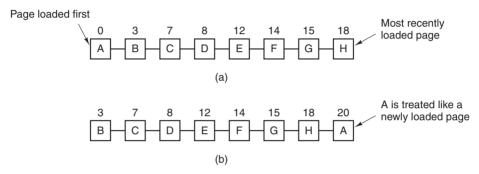
**Figure 3-15.** Operation of second chance. (a) Pages sorted in FIFO order. (b) Page list if a page fault occurs at time 20 and *A* has its *R* bit set. The numbers above the pages are their load times.
