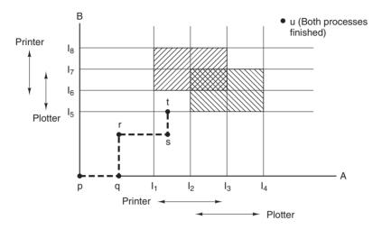
Figure 6-8. Two process resource trajectories.
