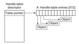
**Figure 11-16.** Handle table data structures for a minimal table using a single page for up to 512 handles.
