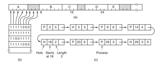
**Figure 3-6.** (a) A part of memory with five processes and three holes. The tick marks show the memory allocation units. The shaded regions (0 in the bitmap) are free. (b) The corresponding bitmap. (c) The same information as a list.
