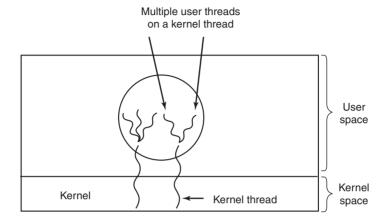
Figure 2-17. Multiplexing user-level threads onto kernel-level threads.
