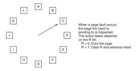
**Figure 3-16.** The clock page replacement algorithm.
