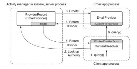
Figure 10-61. Interacting with a content provider.
