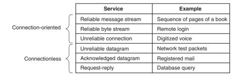
Figure 8-30. Six different types of network service.
