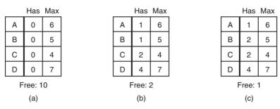
Figure 6-11. Three resource allocation states: (a) Safe. (b) Safe. (c) Unsafe.
