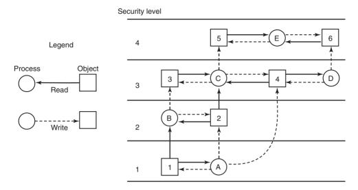
Figure 9-11. The Bell-LaPadula multilevel security model.
