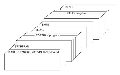
Figure 1-4. Structure of a typical FMS job.
