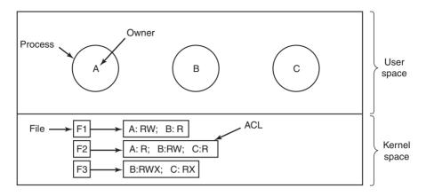
Figure 9-6. Use of access control lists to manage file access.
