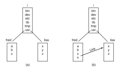
Figure 10-24. (a) Before linking. (b) After linking.
