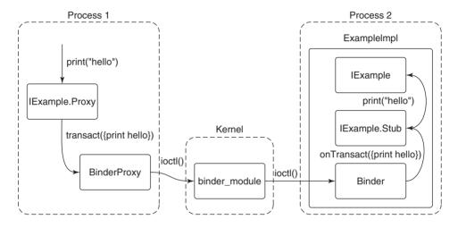
Figure 10-49. Full path of an AIDL-based Binder IPC.
