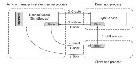
Figure 10-59. Binding to an application service.
