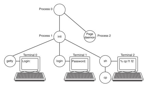
Figure 10-11. The sequence of processes used to boot some Linux systems.
