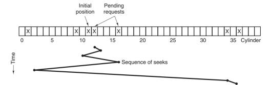
Figure 5-24. Shortest Seek First (SSF) disk scheduling algorithm.
