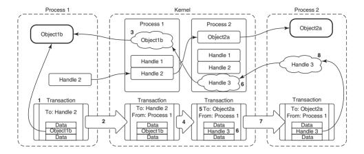
Figure 10-45. Transferring Binder objects between processes.
