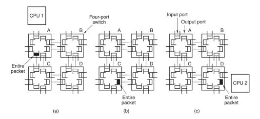
Figure 8-17. Store-and-forward packet switching.
