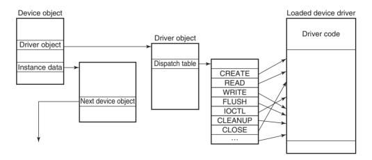
Figure 11-36. A single level in a device stack.
