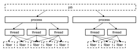
**Figure 11-22.** The relationship between jobs, processes, threads, and fibers. Jobs and fibers are optional; not all processes are in jobs or contain fibers.
