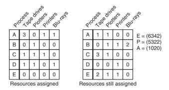
Figure 6-12. The banker's algorithm with multiple resources.
