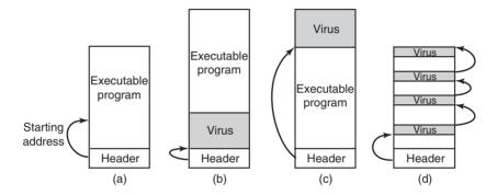
**Figure 9-29.** (a) An executable program. (b) With a virus at the front. (c) With a virus at the end. (d) With a virus spread over free space within the program.
