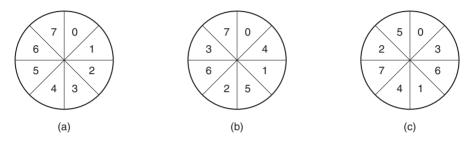
Figure 5-23. (a) No interleaving. (b) Single interleaving. (c) Double interleaving.
