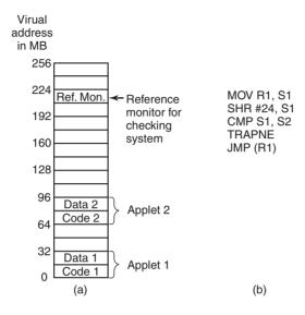
**Figure 9-38.** (a) Memory divided into 16-MB sandboxes. (b) One way of checking an instruction for validity.
