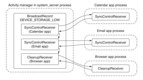
Figure 10-60. Sending a broadcast to application receivers.
