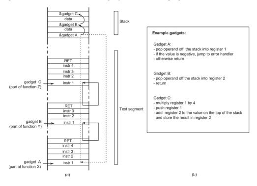
Figure 9-23. Return-oriented programming: linking gadgets.
