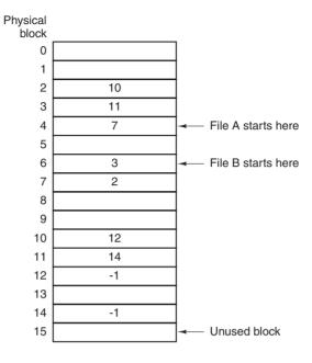
Figure 4-12. Linked-list allocation using a file-allocation table in main memory.
