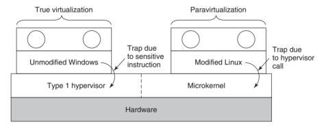
Figure 7-5. True virtualization and paravirtualization
