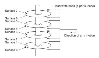
Figure 1-10. Structure of a disk drive.
