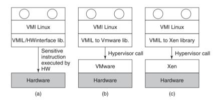
Figure 7-6. VMI Linux running on (a) the bare hardware, (b) VMware, (c) Xen
