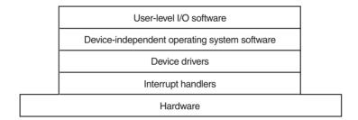
Figure 5-11. Layers of the I/O software system.
