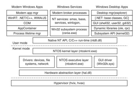
Figure 11-4. The programming layers in Modern Windows.
