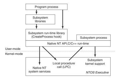
Figure 11-5. The components used to build NT subsystems.
