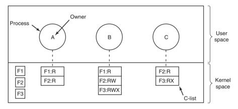
Figure 9-8. When capabilities are used, each process has a capability list.
