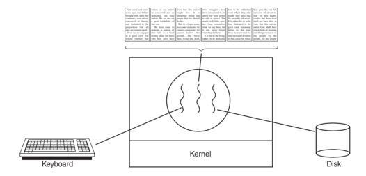
Figure 2-7. A word processor with three threads.
