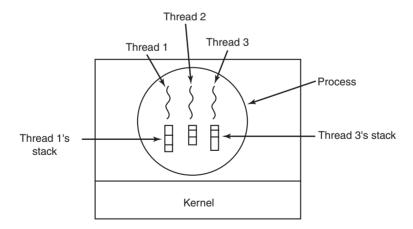
Figure 2-13. Each thread has its own stack.
