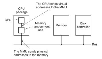
**Figure 3-8.** The position and function of the MMU. Here the MMU is shown as being a part of the CPU chip because it commonly is nowadays. However, logically it could be a separate chip and was years ago.
