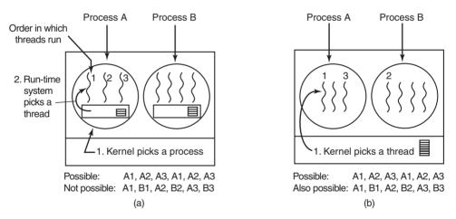
**Figure 2-44.** (a) Possible scheduling of user-level threads with a 50-msec process quantum and threads that run 5 msec per CPU burst. (b) Possible scheduling of kernel-level threads with the same characteristics as (a).
