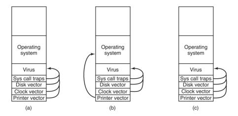
**Figure 9-30.** (a) After the virus has captured all the interrupt and trap vectors. (b) After the operating system has retaken the printer interrupt vector. (c) After the virus has noticed the loss of the printer interrupt vector and recaptured it.
