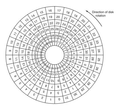
Figure 5-22. An illustration of cylinder skew.
