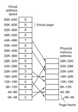
**Figure 3-9.** The relation between virtual addresses and physical memory addresses is given by the **page table**. Every page begins on a multiple of 4096 and ends 4095 addresses higher, so 4K–8K really means 4096–8191 and 8K to 12K means 8192–12287.
