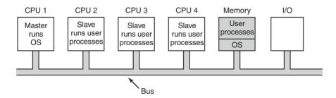
Figure 8-8. A master-slave multiprocessor model.
