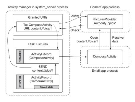
Figure 10-65. Sharing a picture using a content provider.
