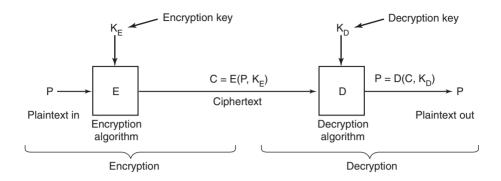
Figure 9-15. Relationship between the plaintext and the ciphertext.
