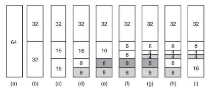
Figure 10-17. Operation of the buddy algorithm.
