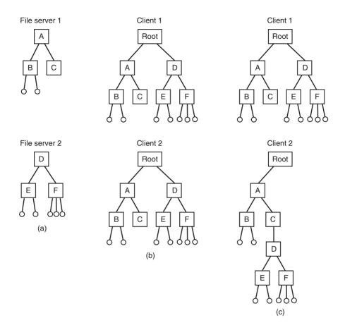
**Figure 8-34.** (a) Two file servers. The squares are directories and the circles are files. (b) A system in which all clients have the same view of the file system. (c) A system in which different clients have different views of the file system.
