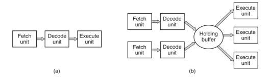
Figure 1-7. (a) A three-stage pipeline. (b) A superscalar CPU.
