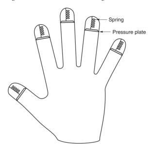
Figure 9-20. A device for measuring finger length.
