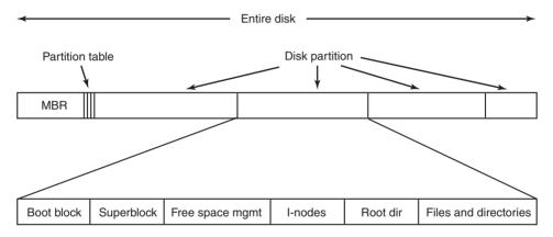
Figure 4-9. A possible file-system layout.
