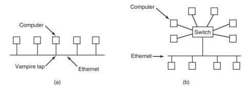
Figure 8-28. (a) Classic Ethernet. (b) Switched Ethernet.
