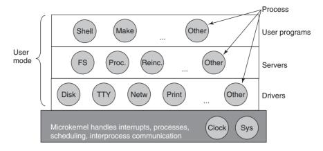
Figure 1-26. Simplified structure of the MINIX system.
