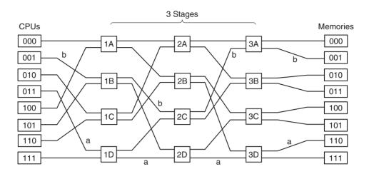
Figure 8-5. An omega switching network.
