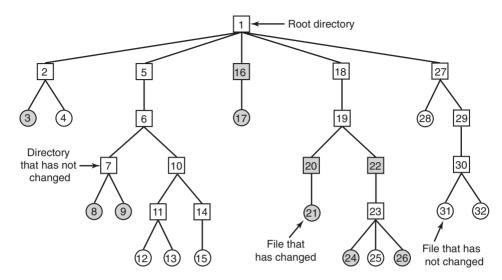
**Figure 4-25.** A file system to be dumped. The squares are directories and the circles are files. The shaded items have been modified since the last dump. Each directory and file is labeled by its i-node number.
