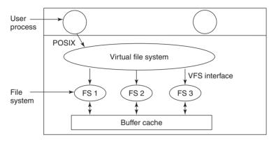
Figure 4-18. Position of the virtual file system.
