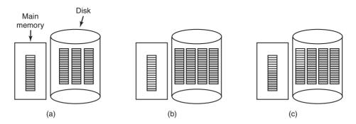
**Figure 4-23.** (a) An almost-full block of pointers to free disk blocks in memory and three blocks of pointers on disk. (b) Result of freeing a three-block file. (c) An alternative strategy for handling the three free blocks. The shaded entries represent pointers to free disk blocks.
