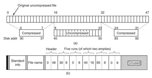
**Figure 11-44.** (a) An example of a 48-block file being compressed to 32 blocks. (b) The MFT record for the file after compression.
