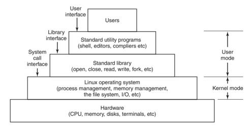
**Figure 10-1.** The layers in a Linux system.
