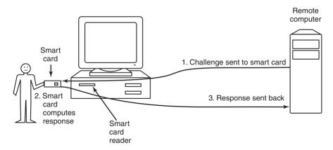
Figure 9-19. Use of a smart card for authentication.
