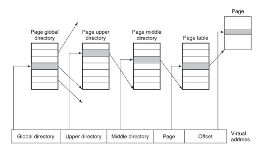
Figure 10-16. Linux uses four-level page tables.
