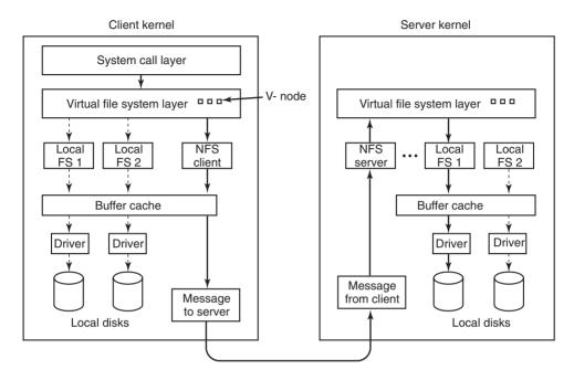
Figure 10-36. The NFS layer structure
