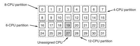
**Figure 8-13.** A set of 32 CPUs split into four partitions, with two CPUs available.
