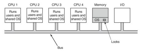
Figure 8-9. The SMP multiprocessor model.
