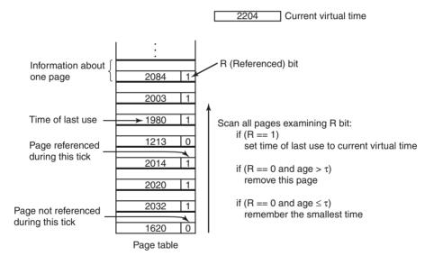
Figure 3-19. The working set algorithm.
