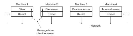
Figure 1-27. The client-server model over a network.
