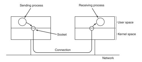
Figure 10-19. The uses of sockets for networking.
