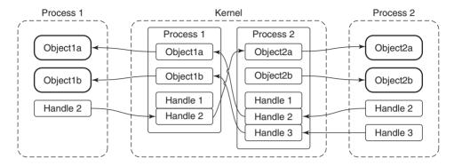
Figure 10-44. Binder cross-process object mapping.
